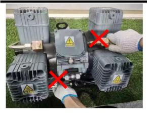
**3.1.5** There is strictly prohibited to pull and handle into/out of the air pipe of Air compressor in carrying in the process of installation, which will lead to deformation or fracture of the inlet/out pipe and affect the performance of the machine.
